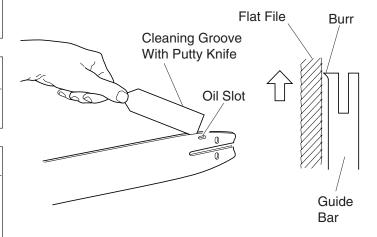
Figure 19 - Guide Bar Maintenance
